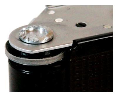
Your A70 will now accept perforated 70mm, non-perforated 70mm, and 65mm motion picture film, as <u>sold by Mercury Works</u>. When using 65mm film, you'll need Mercury "offset" cassette spools. Load your film onto these and then place them inside your Hasselblad A70 insert, with the thin end of the spool facing upward. This positions the film so that it will make full contact with the all-perf wheel in the back.
