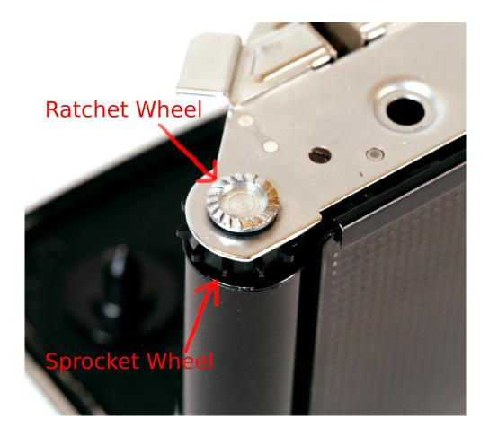
**Step 2: Remove the sprocket wheel from the back.** It isn't anchored once the ratchet wheel has been removed. Also take care to extract the small brass washer that is often installed on top of the sprocket wheel.
