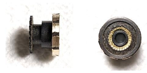
4. Press fit the Mercury plastic ring around the wheel. If it doesn't fit, grind a bit more off the wheel until it does. If it ends up fitting too loosely, fill any gaps with glue. Otherwise, no glue is necessary: ideally this should be a tight friction fit.
