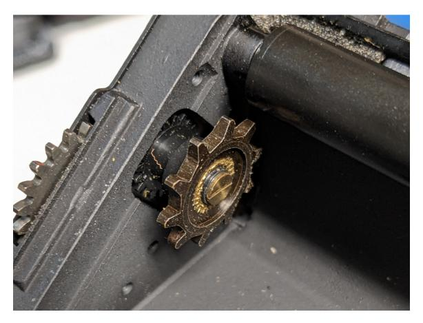
3. Use a bench grinder (best), rotary tool with grinding or cut-off bit, or diamond file to grand off all sprocket teeth. The goal is to produce a round wheel with no protrusions.
