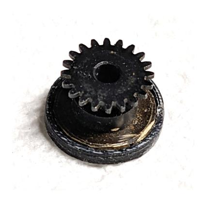
5. Use E6000 glue, applied in a circle around the outer edge of the black plastic. Apply evenly and slowly. It is recommended to apply in two coats. The goal is to end up with a ring of glue about 0.7mm thick, evenly around the plastic:
